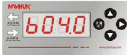
Fig.1 Pre-alarm point setting
